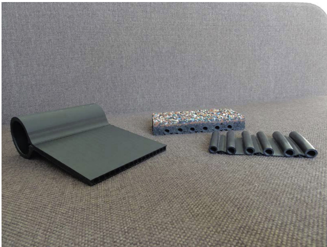
FIGURE 7.16 Samples of panel and strip types of unglazed collectors—solar absorbers.
