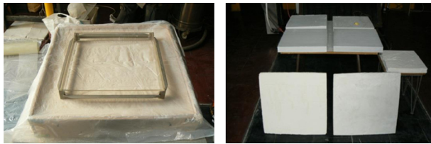
FIGURE 5.19 Composite created of a plasterboard with incorporated PCM made for laboratory testing at the Institute of Heat Engineering, Warsaw University of Technology, Poland. (Photo: R. Wnuk.)
