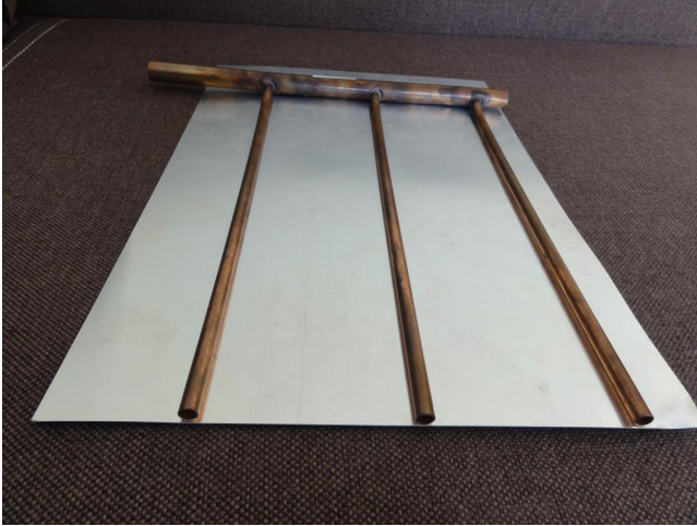
FIGURE 7.13 A sample of a panel absorber (back side).
